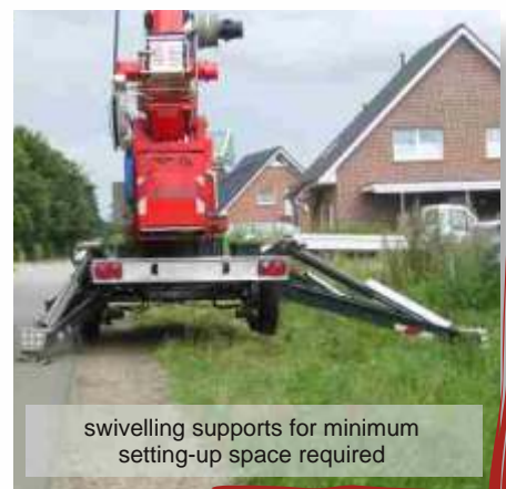
variable folding supports allow extreme ground clearance at the highest degree of safety
